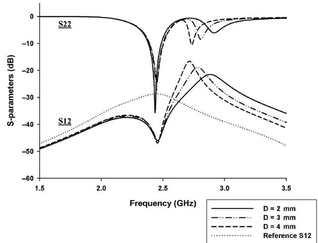
Fig. 7. Simulated parametric study: S-parameters versus frequency for various values of  $D$ .
