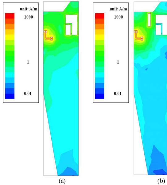
Fig. 3. Simulated surface current distributions upon 2.45-GHz excitation of port 1. (a) Reference design. (b) Proposed design.
