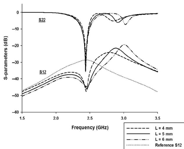
Fig. 8. Simulated parametric study: S-parameters versus frequency for various values of  $L$ .
