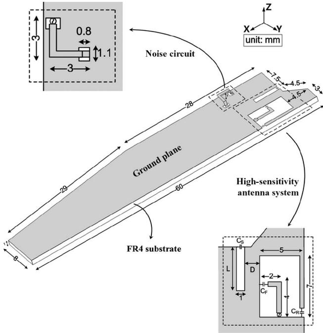
Fig. 1. Geometries of the proposed high-sensitivity antenna system in the PCB ground of a Bluetooth headset.
