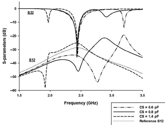
Fig. 6. Simulated parametric study: S-parameters versus frequency for various values of  $C_S$ .
