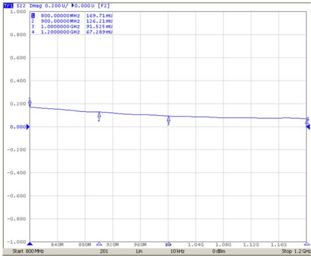
Figure 9 Measurement result of non-Foster reactance. [Color figure can be viewed in the online issue, which is available at wileyonlinelibrary.com ]
